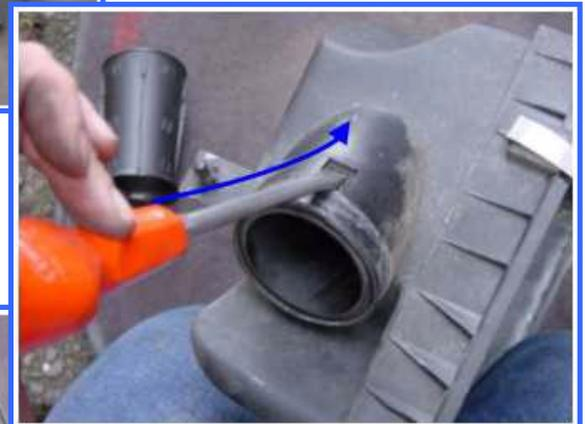
Then pull and 'wiggle' the pipe from the inside to remove it completely.
