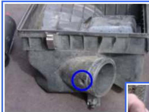
Put a large screwdriver in the hole and push firmly to release the lug, pushing it into the airbox.
