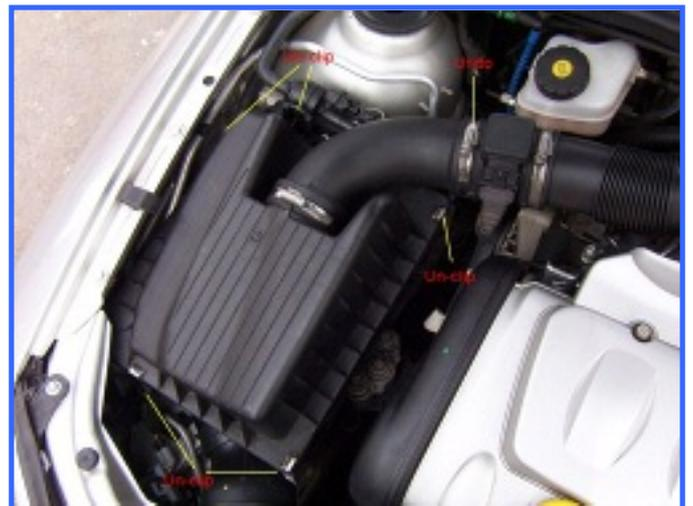
Then by pulling forward the lower half of the air box it comes away from its mountings. Remove from car.
